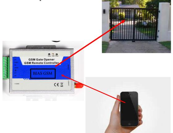
This simple easy to use programmable GSM unit can be installed to operate you roller door or auto gate just install a sim card then program the GSM unit via text message from your mobile.
